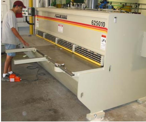
Shop Technician, Brian Shomo , prepares to use the new sheet metal shear. This machine handles material as large as 10' long and 1/4" thick.
