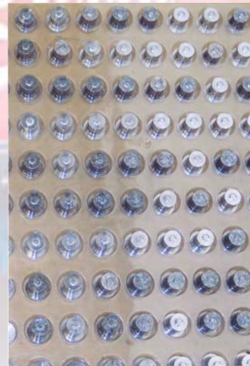
Valve plugs used in fountain drink dispensers undergo an 11-hour hydrogen cleaning process at San Antonio.
